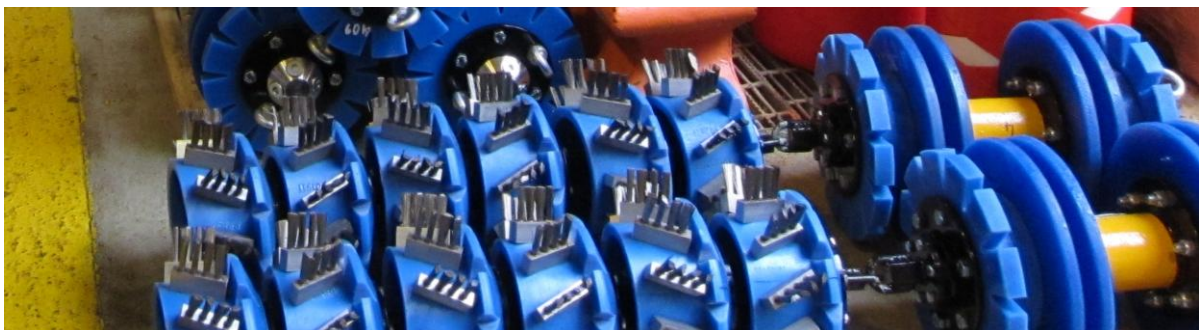
Figure 11. Brush pigs for removing debris.
