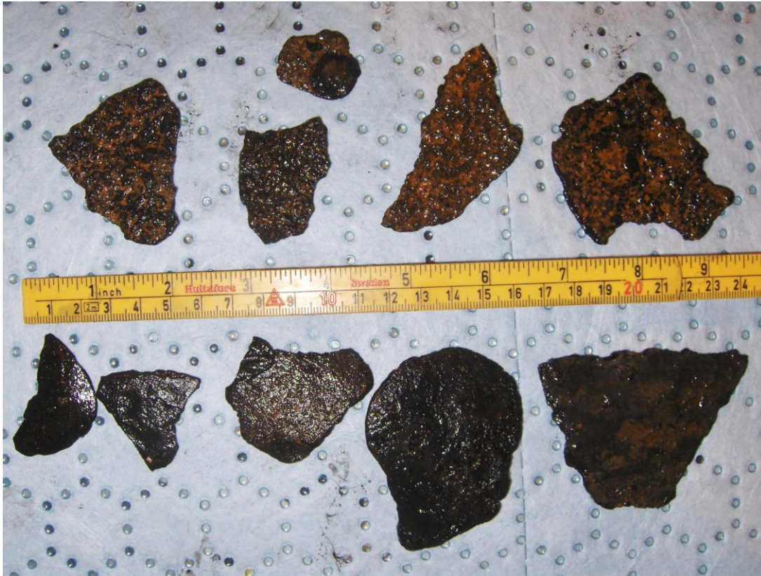
Figure 3. Picture shows debris flushed out of the pipeline prior to launching pig no. 1 in October 2010
