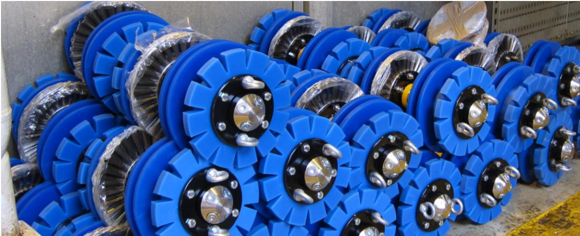
Figure 13. Cleaning pigs for removing scale.
