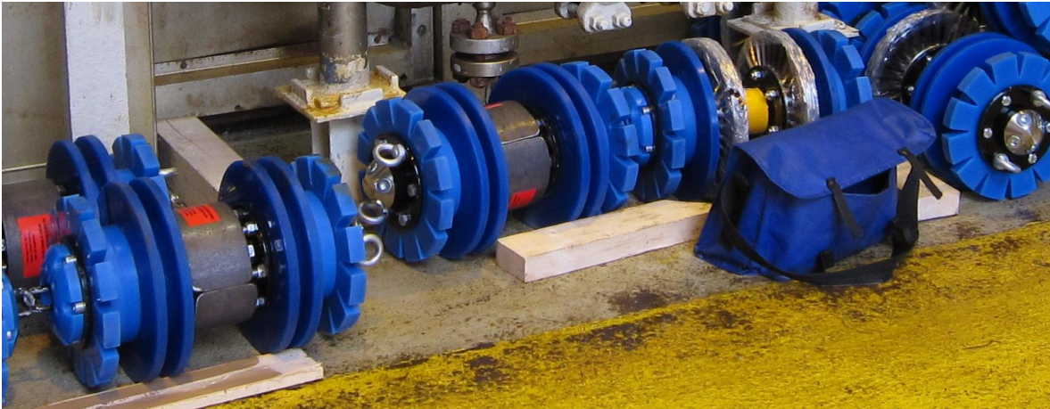
Figure 14. Pigs with magnets to remove magnetic debris.
