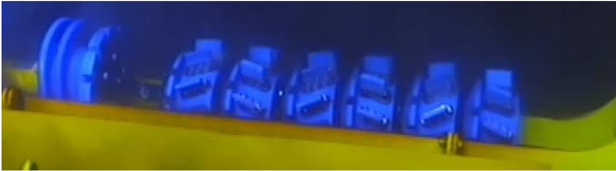
Figure 12. Scraper pig for removing scale.
