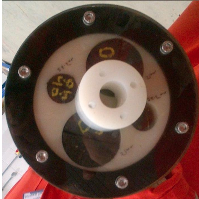
Figure 4 – Carrier spool and rods used in testing
