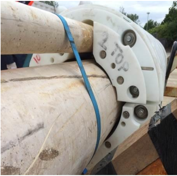
Figure 6 – Five layer PP insulated pipe with piggyback line
