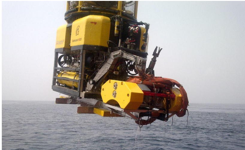
Figure 11: The MEC™-Combi Crawler on site.
