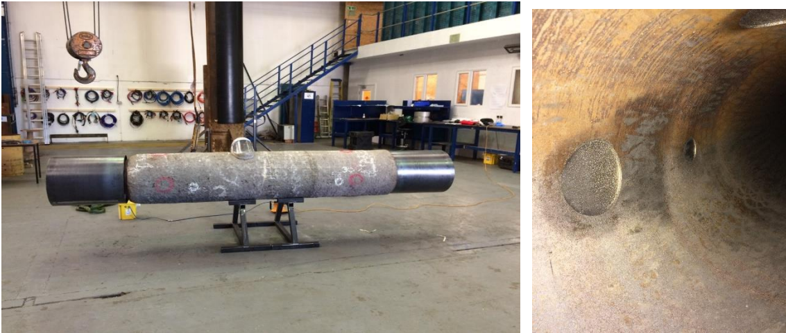
Figure 7: Concrete weight coated test spool (left) and example of artificial defect (right)
