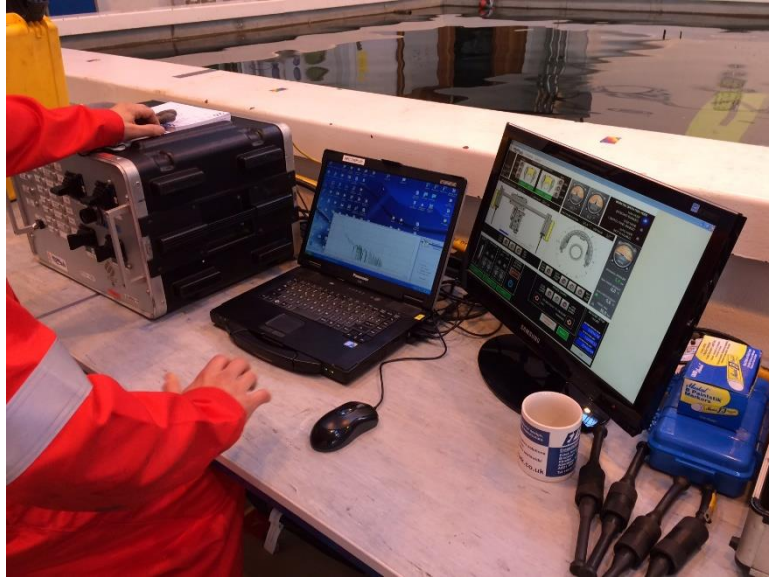
Figure 9: Control Box, data visualisation software and subsea tool control software
