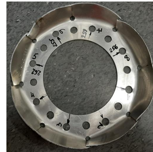
Cup shaped damage could be associated with a 360° reduction. For example a reduced bore valve
