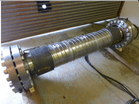
Pipe burst tests to 1700psi
