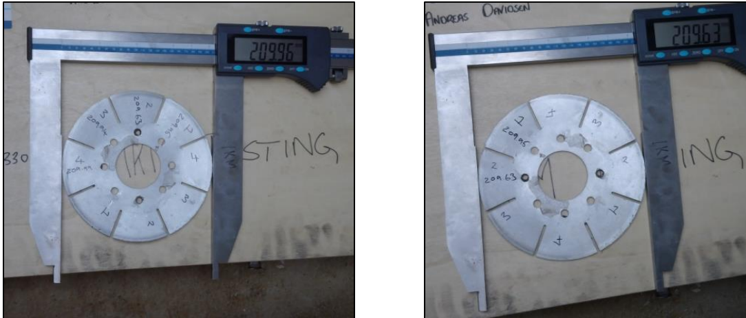
Figure 11 - 2019 Inspection Gauge Plate
