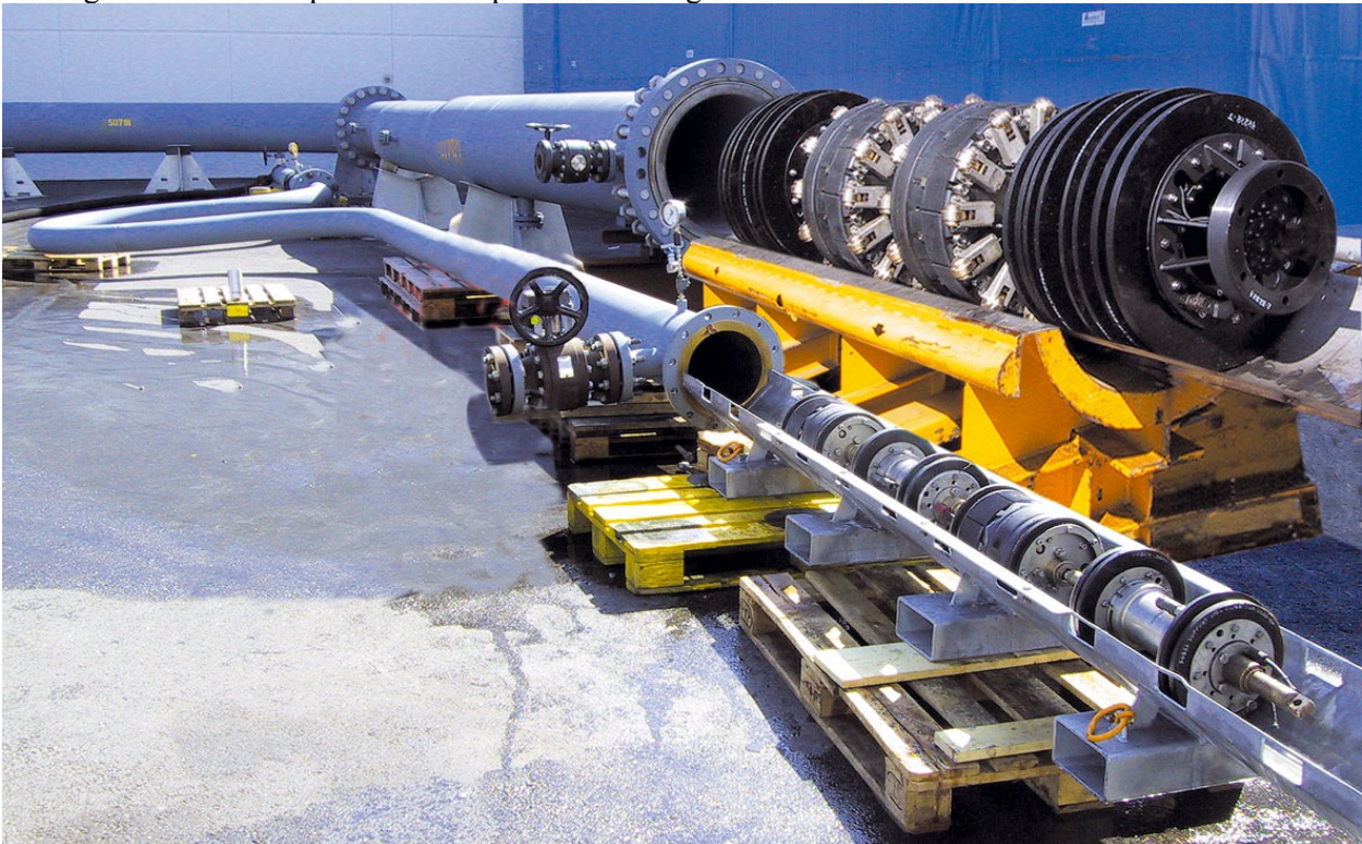
Figure 12. 10 inch and 32-inch piggability test rigs
